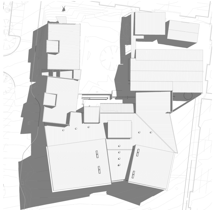
CAD generated 9am 22 September shadow diagram required for double auditorium extension project application
